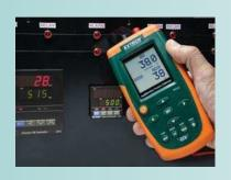
Precision source and measure for thermocouples (8-Types), mA, mV, and V devices
